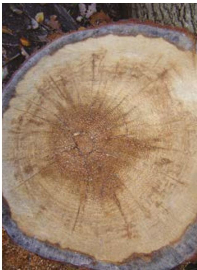
Figure 3 Severe star shake with extensive brown staining present indicating presence of bacterial wetwood (chalky deposits are also visible in these shakes).
