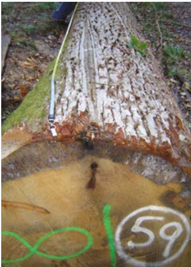
Figure 5 Seam indicating a partially healed frost crack. Note the corresponding split in the wood beneath it. In this instance the dark staining is not thought to be bacterial wetwood and may be associated with a Phytophthora .
